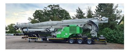
It takes less than an hour to complete the unfolding operation once the unloader arrives on site. Packing away at the end of unloading is equally quick, and these tasks can be carried out by a single operative.
